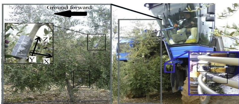
Fig. 10 - Dynamic response analysis test of the olive tree
