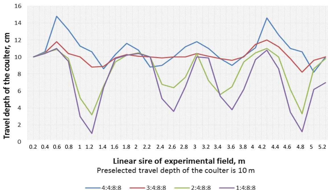
Fig. 8 – The effect of the coulter suspension ratio AB CD BC AD to the uniformity of the coulter travel when passing rough spots
