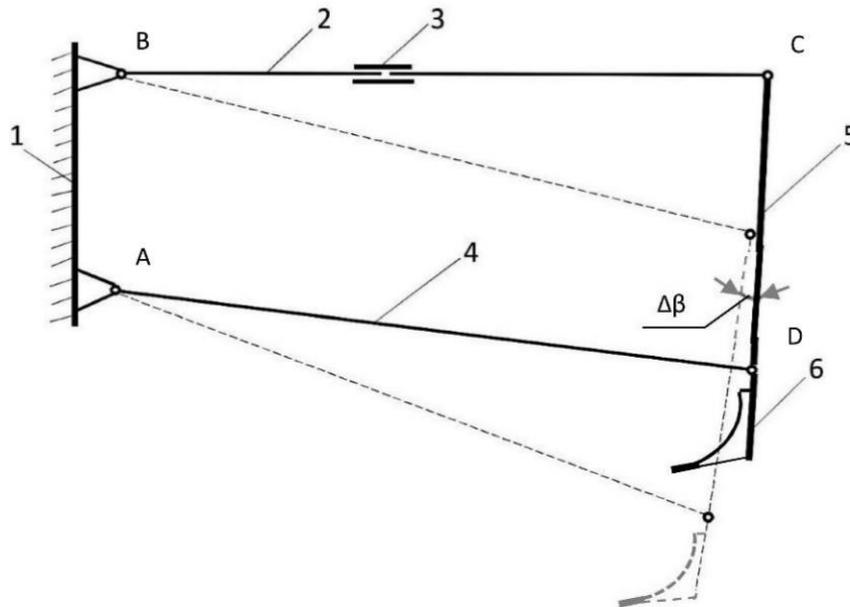
**Fig. 3 – Schematic diagram of the coulters individual floating suspension operation**
