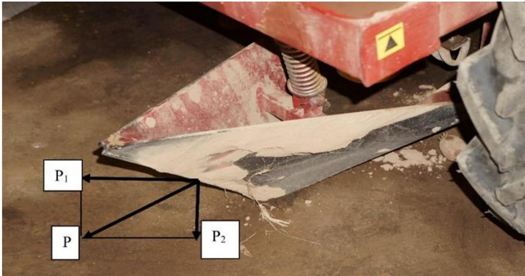
**Fig. 1 – Coulter with a blunt angle of soil entry of L-202 potato planter**
