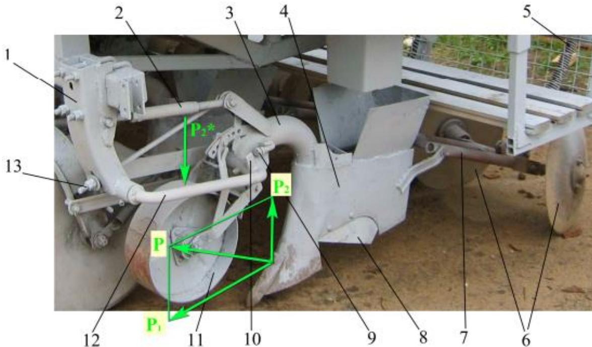
**Fig. 2 – Coulter group of the KSU-4 clone potato planter (VIM)**
