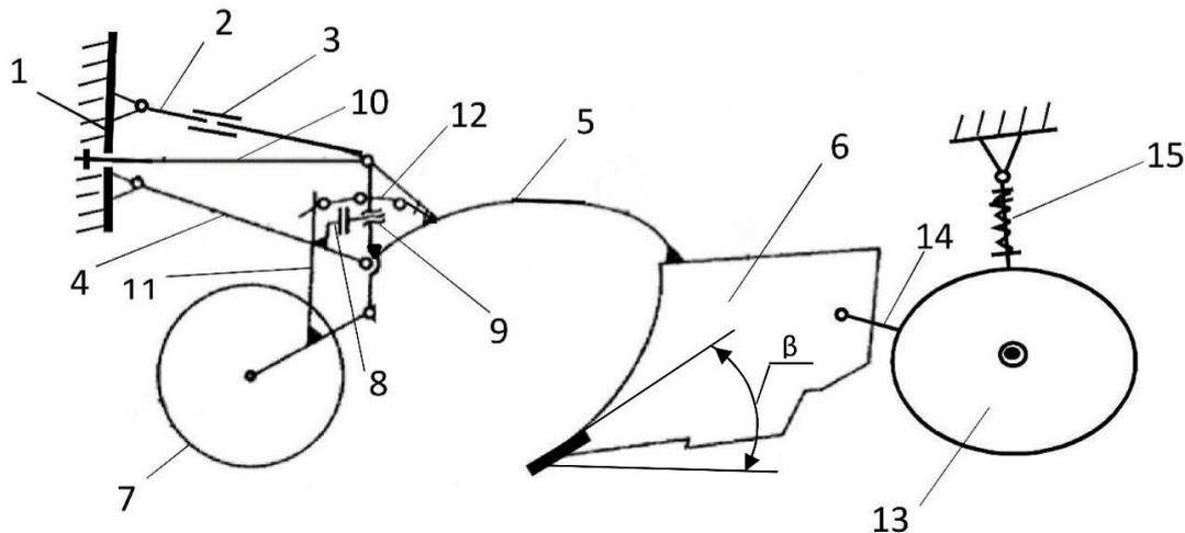
**Fig. 4 – Coulters group of potato planters with automatic stabilization of planting depth**
