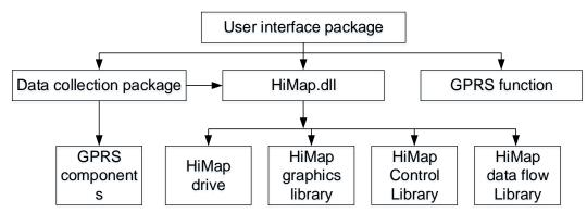
Fig. 3 - The overall mechanism design of data acquisition application software
