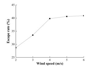
Fig. 5 - Escape rate on the circular sieve as a function of wind speed
