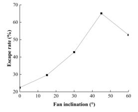
Fig. 6 - Escape rate on the circular sieve as a function of fan inclination
