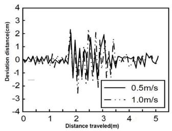
Fig. 5 - Lateral deviation of vehicle circle curve line running at different speeds
