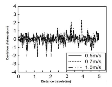
Fig. 4 - Lateral deviation of vehicle running in straight line at different speeds
