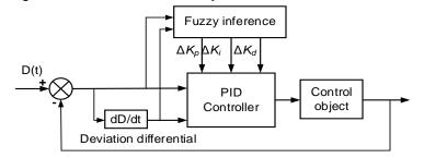
Fig. 1 - Structure diagram of fuzzy PID controller
