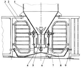
**Fig. 3 - Mechanism of the self-feeder** 1-hopper; 2-pen partition; 3-removable partitions; 4-discharge neck, 5-agitator; 6-slots; 7-flexible suspension; 8-round trough; 9-contact grille
