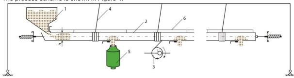
Fig. 4 - The technological scheme of the modernized vibrating feed distributor
