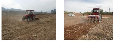
a) 1GQN-200-type rotary tiller b) 2BJY-3-type hard stubble planter Fig. 2 - Materials of the second-period test
