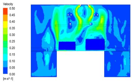
Fig. 15 - Velocity distribution of Y = 0m
