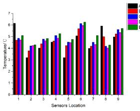
Fig. 11 - Temperature values at height of 1.6m in pigsty (right)
