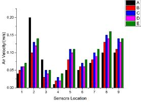
Fig. 8 - Airflow velocity values at height of 1m in pigsty
