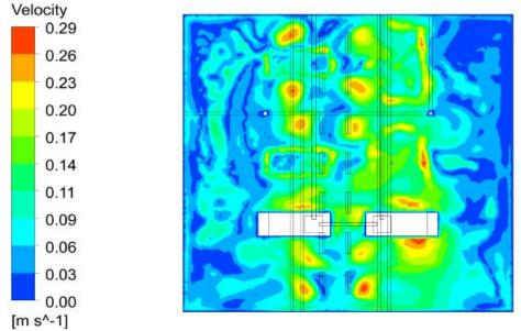
Fig. 14 - Velocity distribution at Z = 0.81m
