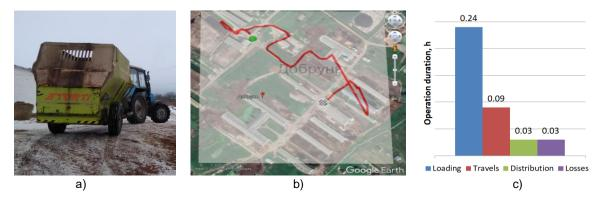
Fig. 2 – Mobile TMR mixer Storti Husky MT 90 (a), Routing track, recorded in mobile application «Strava» (b) and Constituents of time balance of the mobile mixer operating cycle (c)
