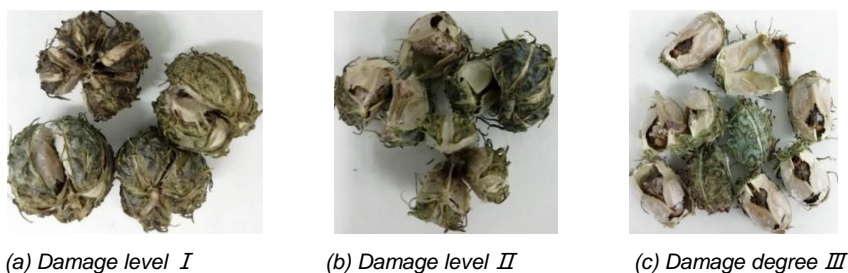
Fig. 14 - Classification of collision damage levels of castor
