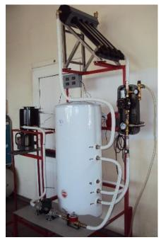
Fig. 2 - Physical development of the combined thermal system experimental model
