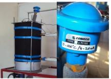
Fig. 7 - Installation of thermal detector to the tank (S4)
