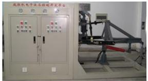
(b) Tractor electro-hydraulic control test bench
