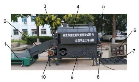
Fig. 4 - Performance experiment unit of buckwheat threshing device 1- Conveyor belt; 2- Feeding bridge; 3- Internal roller reducer; 4- Threshing device; 5- External roller reducer; 6- Control box; 7- Receiving box; 8- Motor of 1.5 kW; 9- Frame; 10- Motor of 7.5 kW
