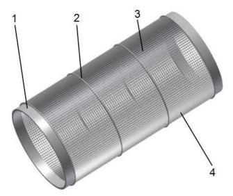
Fig. 3 - Structure of concave grate roller 1- Support drive plate; 2- Ring plate; 3- Rib; 4- Wire ring
