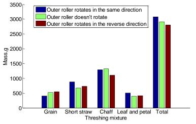
Fig.8 - Mass of components under different outer roller rotation conditions
