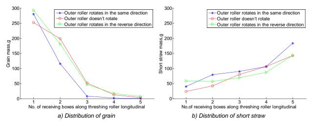
Fig.10 - The components proportion under different conditions of external roller rotate
