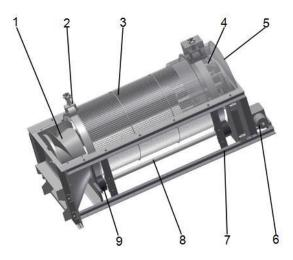
Fig. 1 - Structure of internal and external rotary roller buckwheat threshing device 1- Screw feeding device; 2- Pressing wheel; 3- Concave grate roller; 4- Threshing roller; 5- Top cover; 6- Reducer; 7- Frame; 8- Transmission shaft; 9- Friction wheel
