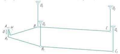
Fig. 1 - Design model of the grain cleaning machine sieve frame
