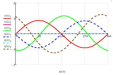
Fig. 5 - Graph of changes in the acceleration (rad/s²) of the links of the grain cleaning machine sieve frame
