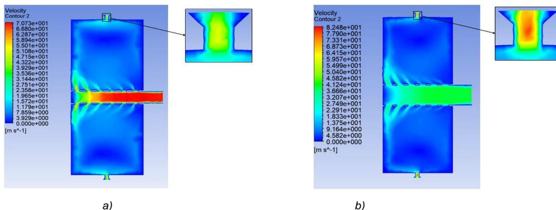
Fig. 3 - Velocity cloud diagram of negative pressure cavity with different tube diameters
