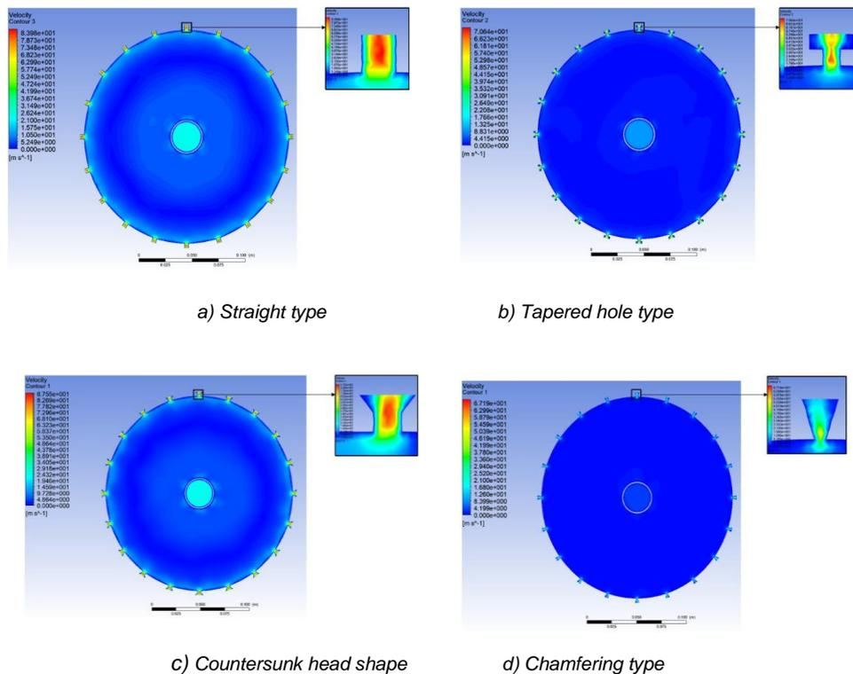
**Fig. 7 - Airflow velocity map under different socket hole**
