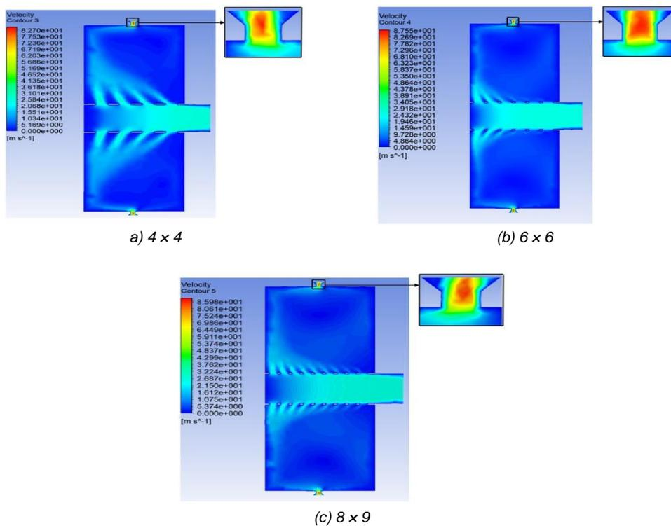
Fig. 5 - Velocity cloud diagram of negative pressure cavity with different vent layout
