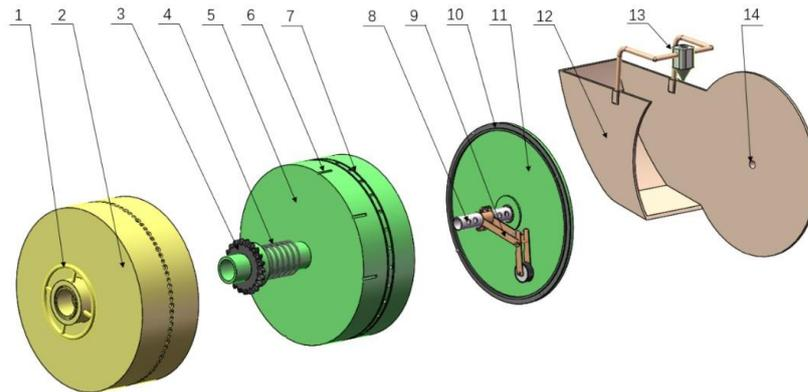
**Fig.1 - Schematic diagram of seed metering device**
