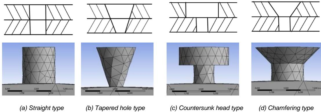
**Fig. 6 - Shape and mesh of socket hole**
