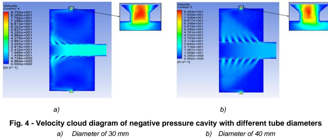
Fig. 4 - Velocity cloud diagram of negative pressure cavity with different tube diameters
