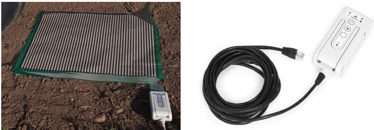
Fig. 2 – Tekscan pressure sensor before testing and VersaTek Handle data acquisition system
