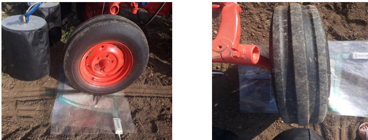
Fig. 4 – Front tire at minimum inflation pressure (100 kPa)
