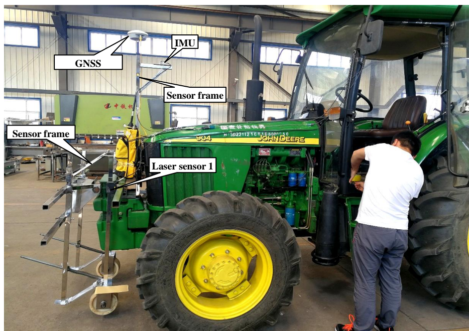
Fig. 1 - Profiling apparatus mounted on the front counterweight of a tractor
