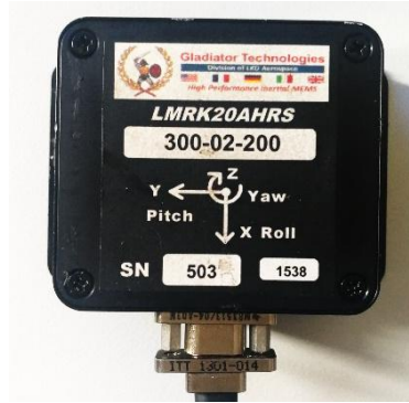
Fig. 7 - Coordinates of x (Roll), y (Pitch) and Z (Yaw) on the IMU
