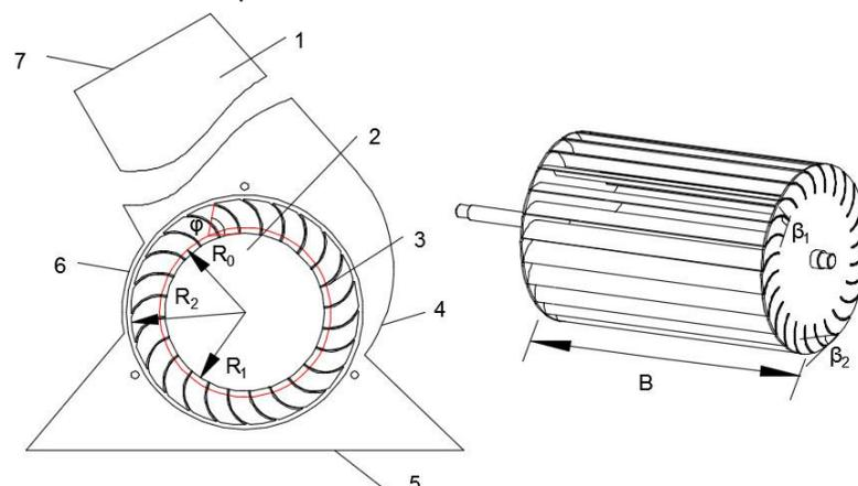
**Fig. 3 - Structure diagram of cross-flow fan**
