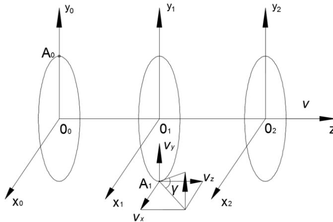
Fig. 9 - Kinematic analysis diagram of peanut pods
