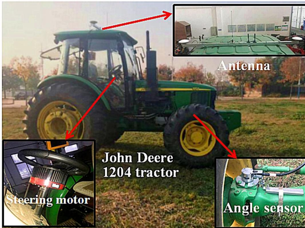
Fig. 3 - Platform of tractor cross-boundary warning system
