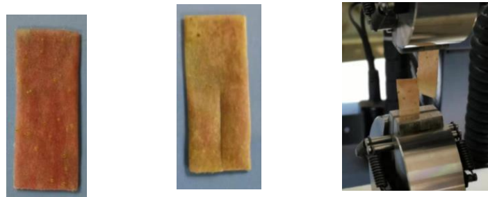
a. Peel sample b. Structure specimen c. tearing test
