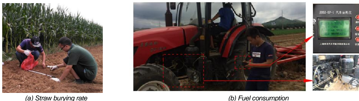
Fig. 11 - Field test measurement
