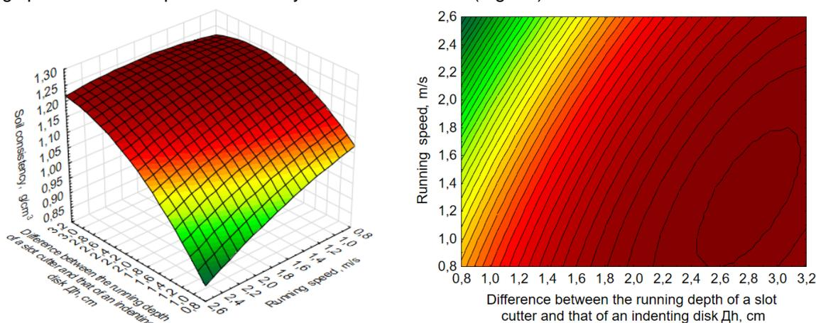
**Fig. 10 - Response surface of the change in soil consistency  $\rho$  depending on the parameter  $\Delta h$  and the running speed  $V$**
