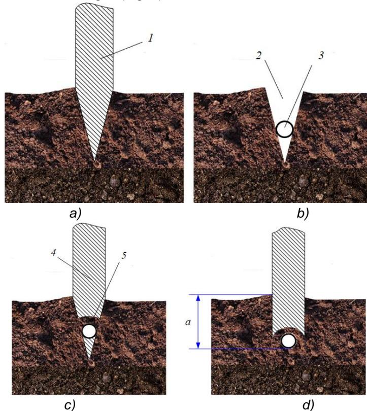
**Fig. 1 - The main stages of two-phase seed covering**
