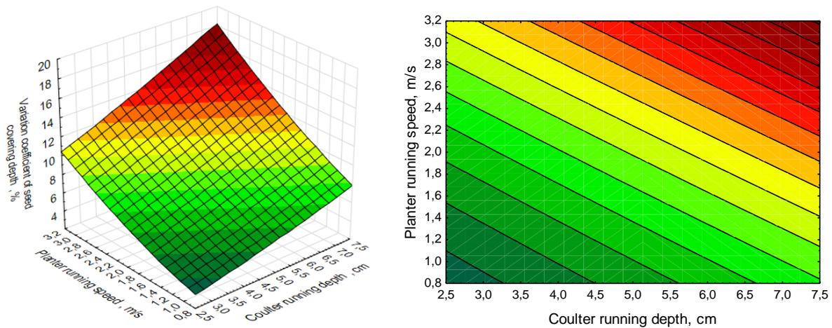
Fig. 11 - Response surface of the variation coefficient of seed covering depth *W* depending on the running speed of a planter *V* and the set running depth of a coulters *H*
