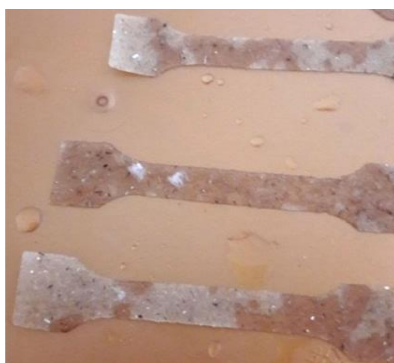
Fig. 1 - Selected test samples after being in a high humidity environment
